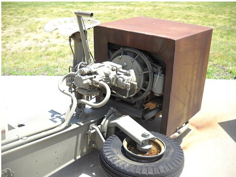
XM123 medium auxiliary propelled 155 mm howitzer seat and power unit at the Rock Island Arsenal Museum.
